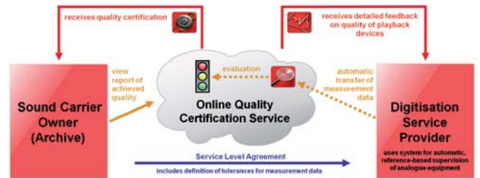
Figure 4. Quality control when digitising analogue media with the help of an online quality certification service.
