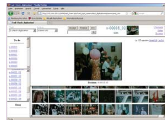
Figure 4. This is the view of the detected shots. It shows some results of the detected cuts and transitions. The larger picture on the top represents the activated thumbnail below. In addition, the application also detects any extant picture errors, interprets them as cuts and creates thumbnails, as it does with all normally detected cuts. Thus, many failures become visible at a glance.
